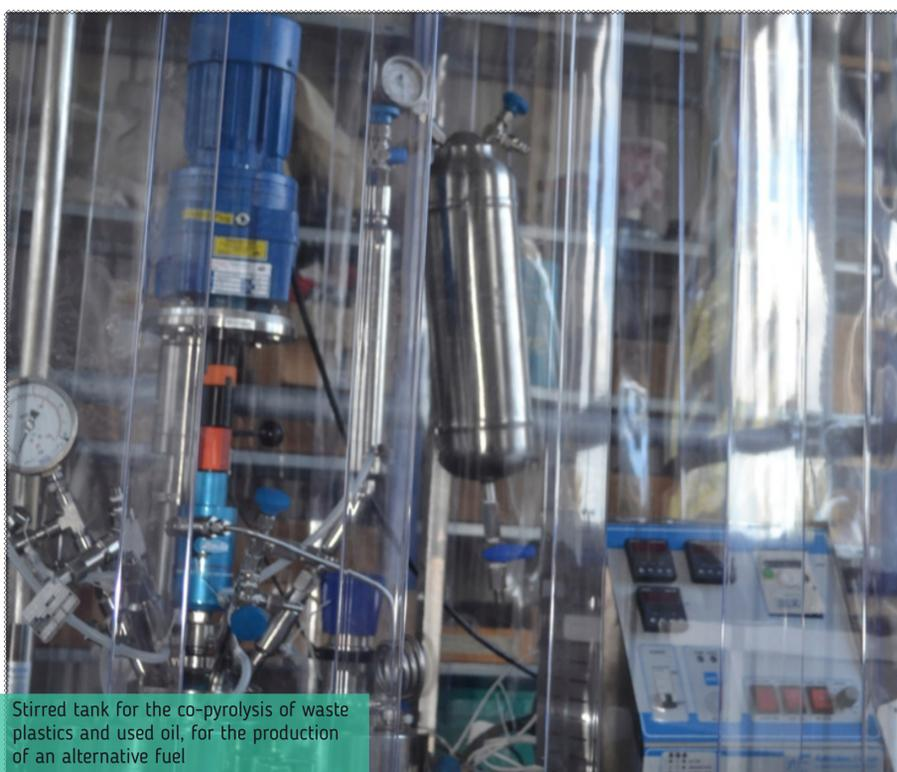
Stirred tank for the co-pyrolysis of waste plastics and used oil, for the production of an alternative fuel
